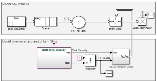
The seExampleTankFilling example has two sections, a SimEvents part that models event-based behavior and a Simulink part that models continuous-time dynamics.
