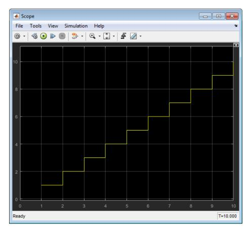
After an entity departs from the Entity Server block, the block updates its output signal at the  ${\bf d}$  port.
