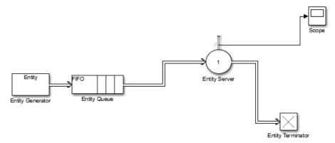
SimEvents connects the source block to the destination block. If necessary, the software also routes the connecting line around intervening blocks or lines.
