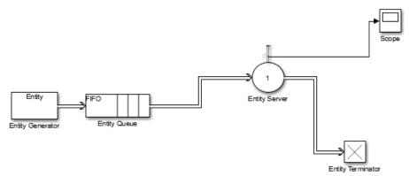
The existence of the entity path does not guarantee that any entity actually uses the path. For example, the simulation could be so short that no entities are ever generated. Even when an entity path is used, it is used only at a discrete set of times during the simulation.
